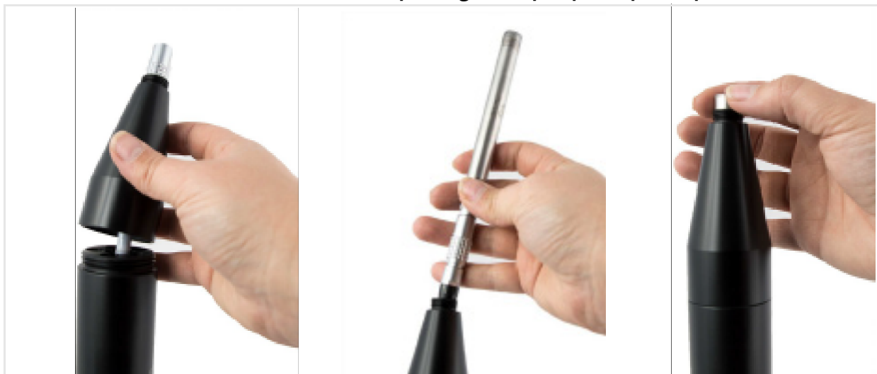
FIGURE 2-3 Replacing the top cap and preamplifier
