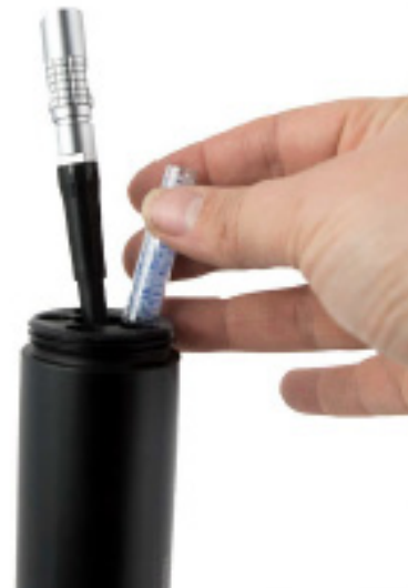
FIGURE 2-2 Replacing desiccant cartridges
